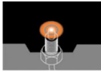
Thermography of flow monitor with no flow. The color graduations around the sensor tip show how the fluid is heated up by the heat source within the flow monitor.
